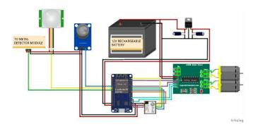
Fig -4: Descriptive Diagram of Robot
