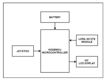
Fig -2: Block Diagram of Remote-control
