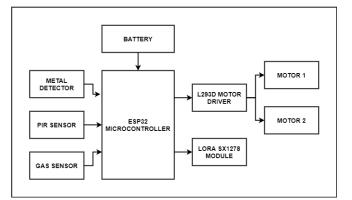
Fig -1: Block Diagram of Robot
