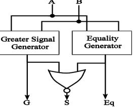
comparator as shown in Figure 3.1 which computes greater and equal in place of greater and smaller. The greater and equal signals are further used to generate the small signal.
