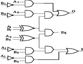
Figure 2: Logical diagram of 2-bit comparator
