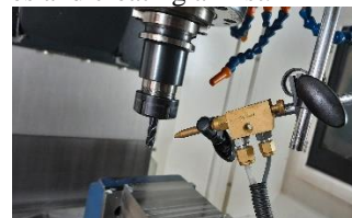
Fig 4.1 Lubricant sprayed in tip of the tool
