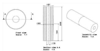
Roller can be considered to be a hollow shaft subjected to torsional load.
