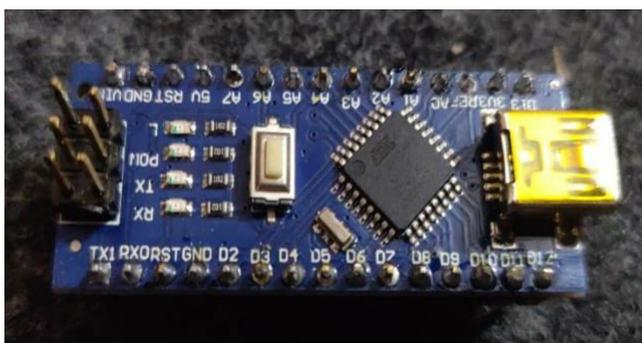
**Fig. 2 : Arduino NANO Based on AtMega-328p**
