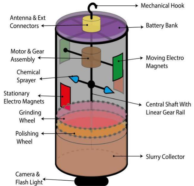
**Fig. 3 : Design of climbing robot**
