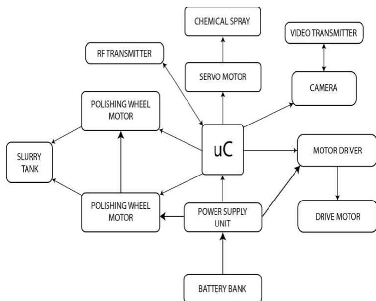
**Fig. 1 : Block diagram of manual operation adjustable robot**
