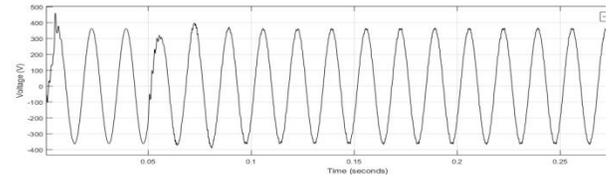
Fig.6.8: Inverter output Voltage with filter
