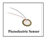
Fig 10. Piezoelectric sensor for Blood Pressure measurement
