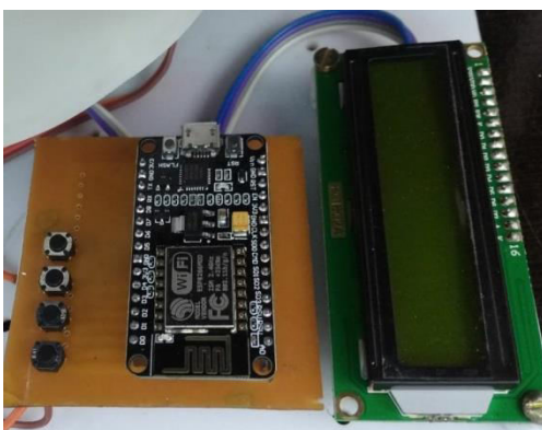
Figure 3.: Medicine Scheduler using NodeMCU
