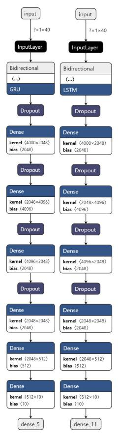
Fig. 4. The architecture of the First and Second Model
