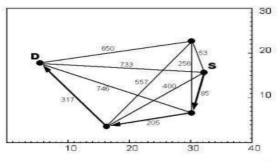
Figure 1: Example of algorithm that finds the minimum energy source-destination path (with  $\alpha = 2$  and  $\mathcal{E}_{max} = 70^2$ ). Shown is the key step, consisting of a graph transformation that we continually refer to this paper as the "Energy Cost Graph". The minimum energy path is highlighted in bold, and has aggregate energy cost 607.
