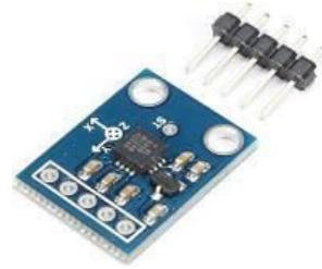
(ADXL 335 THREE AXIS ACCELEROMETER )
