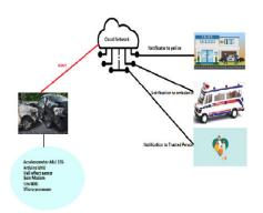
The device is designed in such a way that it immediately detect the Collison using ADXL 335 accelerometer with raspberry pi 3B+.
