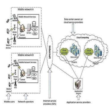
**Figure 2: Building of Mobile Cloud Computing** (MCC)
