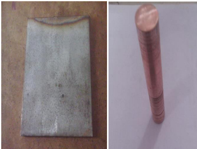
Fig2: Grade E 304 Stainless Steel (Work Piece) And Copper (Tool)
