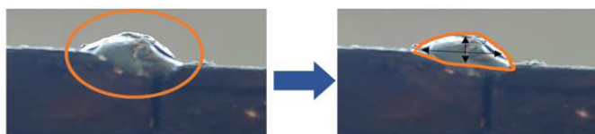
Fig. 2. Actual weld bead of metal arc welding.
