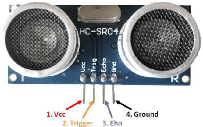
Fig-4: Ultrasonic Sensor
