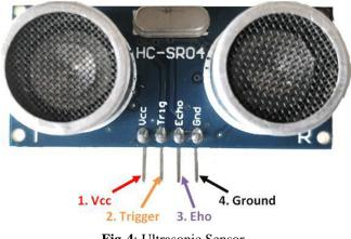
Fig-4: Ultrasonic Sensor
