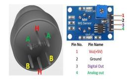
Fig 7. MQ-2 Sensor
