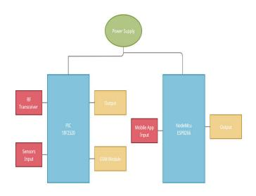
Fig 1. Block diagram of Multiple Sensors fault detection and monitoring system using PIC, GSM, and IoT
