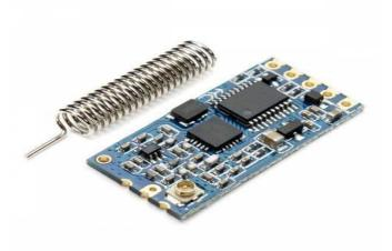
Fig 8. HC12 RF Transceiver module
