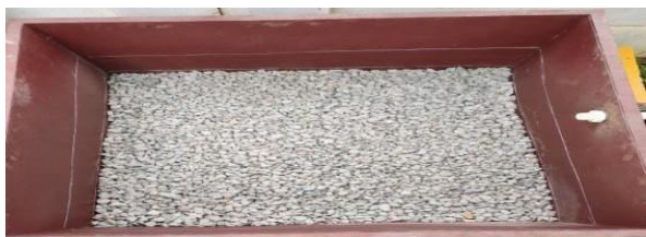
Fig7.1.3: showing the bottom second layer filled with 12 mm aggregate
