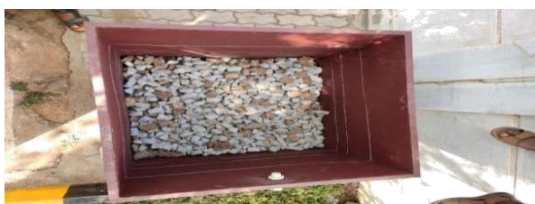
Fig7.1.2 : showing the bottom layer filled with 40mm aggregates
