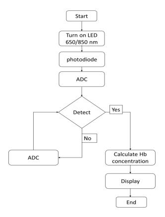
Fig. B: Flow chart of the system
