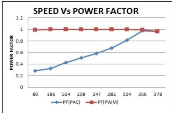
Fig. 10 speed V/s power factor
