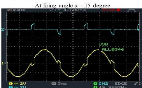
Fig.2 Blue waveform shows voltage across switch (Vsw)
