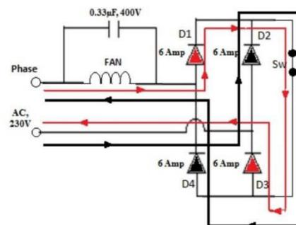
Fig.5 Conduction mode
