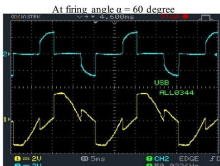
Fig.3 Blue waveform shows voltage across switch (Vsw)
