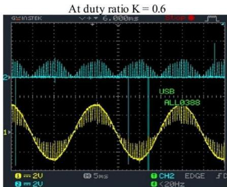
Fig. 7 Blue waveform shows voltage across switch (Vsw)
