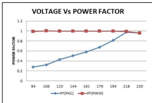
Fig.11 Voltage Vs Power factor
