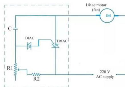
Fig.1. Phase Angle control fan regulator
