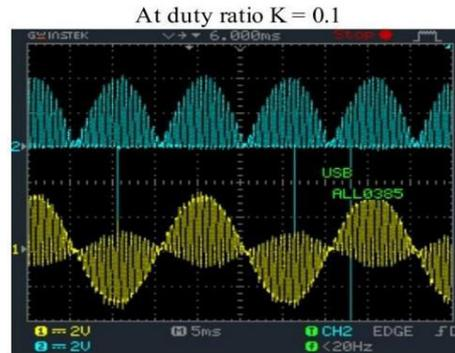
fig. 9 Blue waveform shows voltage across switch (Vsw)
