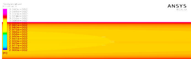
Fig -7:Temperature distribution near outlet of the pipe for Re = 10000, A = 0.1, f = 0.4
