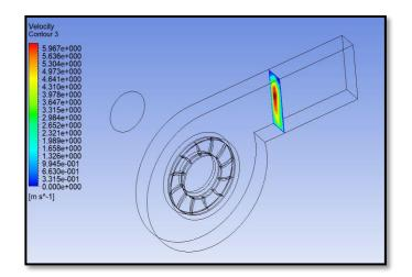
Fig.3(a). Outlet Velocity Plot
