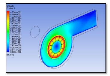
Fig.3(b). Overall Velocity Plot
