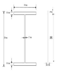
Fig(1): Cross sectionFig(2): Cross section details of steel beam details of notch
