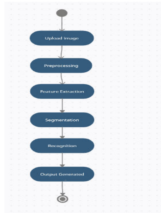
Fig -3.4: Sequence diagram of the text recognition process
