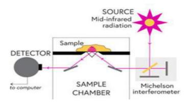
Fig-1:Block Diagram Of Mir Spectroscopy
