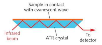
Fig-2: Attenuated Total Reflection
