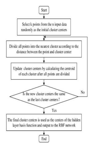
Figure-5: Flow Chart of K-Means Clustering
