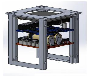
Figure 3. Slotted rack and dummy payloads
