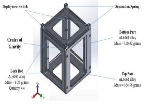
Figure 1. CubeSat Structure
