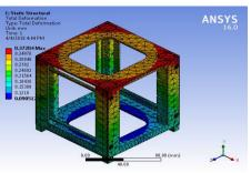
Figure 5(a). Total deformation
