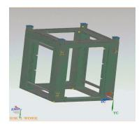
Figure 4. Fix Support in software analysis
