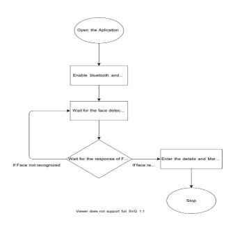
Like the workflow suggests, the application uses a raspberry pie device as a bluetooth peripheral to verify the location of the student (user). It only proceeds upon verification.
