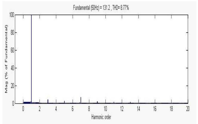
Fig -19: THD with R-L Load Using PD Technique
