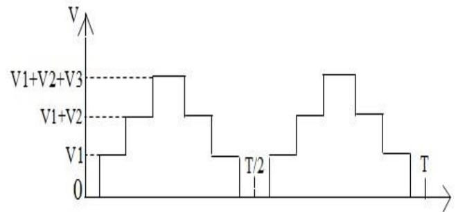
Fig -7: Unipolar 7-Level Voltage Output
