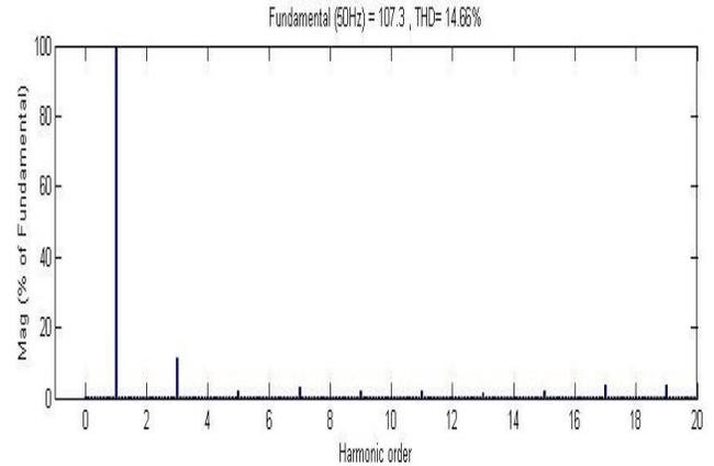
Fig -23: THD with R-L Load Using APOD Technique
