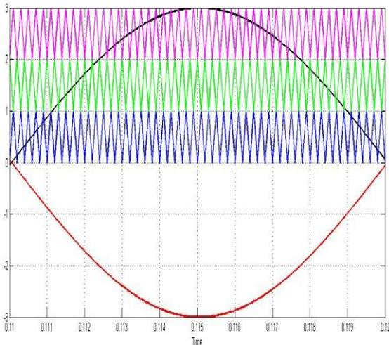
Fig -10: Carrier Arrangements for APOD PWM Technique
