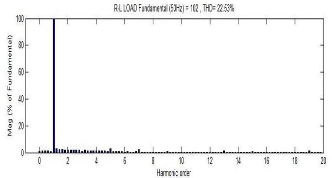
Fig -18: THD with R Load Using PD Technique
