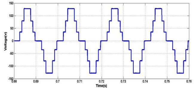
Fig -12:7-Level Inverter Voltage Output with R Load
