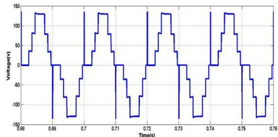
Fig -13:7-Level Inverter Voltage Output with R-L Load
