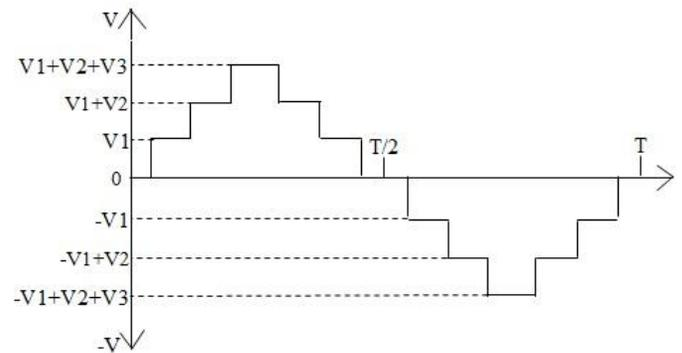
Fig -8: Bipolar 7-Level Voltage Output
