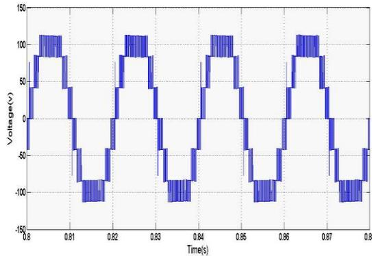
Fig -21: Output Voltage with R-L Load using APOD Technique
