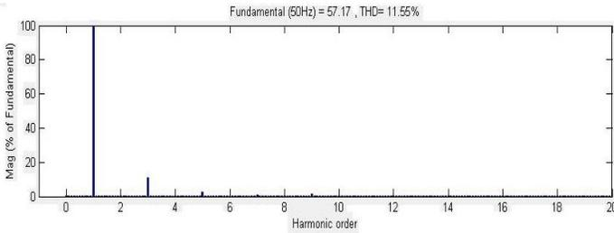
Fig -15: THD with R-L Load Using SPWM Technique
