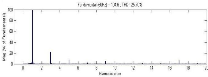
Fig -14: THD with R Load Using SPWM Technique
