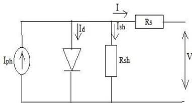
Fig -2: Equivalent circuit of PV cell
