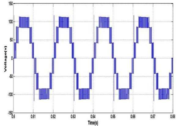
Fig -17: Output Voltage with R-L Load Using PD Technique
