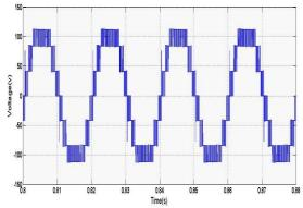
Fig -21: Output Voltage with R-L Load using APOD Technique
