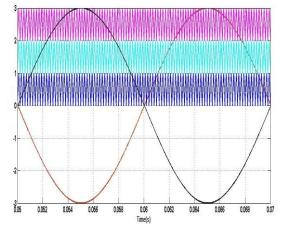
Fig -9: Carrier Arrangement for PD PWM Technique
