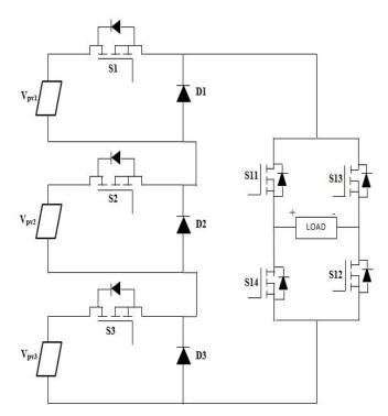
Fig -4: Circuit Diagram of DC-Link H-Bridge Inverter
