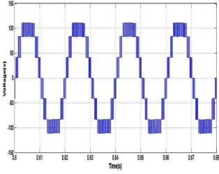
Fig -16: Output Voltage with R Load Using PD Technique
