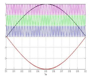
Fig -10: Carrier Arrangements for APOD PWM Technique
