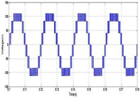
Fig -20: Output Voltage with R Load using APOD Technique
