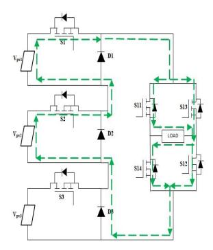
Fig -6: Mode of Operation When S2 Is ON
