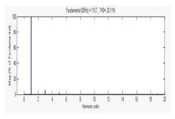
Fig -22: THD with R Load Using APOD Technique
