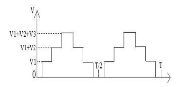
Fig -7: Unipolar 7-Level Voltage Output
