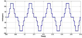
Fig -12:7-Level Inverter Voltage Output with R Load
