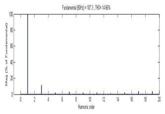
Fig -23: THD with R-L Load Using APOD Technique
