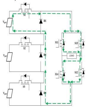
Fig -5: Mode of Operation When S1 Is On
