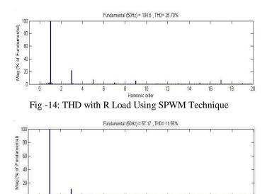
Fig -15: THD with R-L Load Using SPWM Technique
