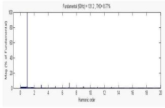
Fig -19: THD with R-L Load Using PD Technique
