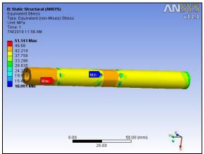
Fig.4.c Evaluating Equivalent Stresses
