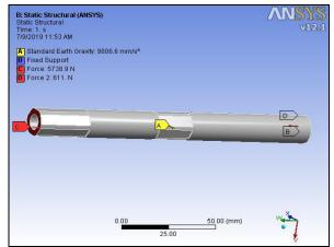
Fig.4.a Applying Boundary Conditions
