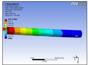
**Fig.4.e** (ii) Natural frequencies at 2<sup>nd</sup> node.
