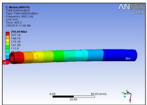
Fig.4.e (i) Natural frequencies at 1<sup>st</sup> node.
