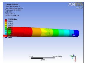
Fig.4.e (v) Natural frequencies at 5<sup>th</sup> node.
