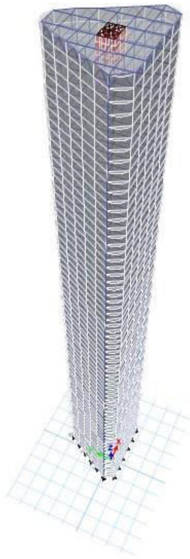
Figure 4.3: 3 – Dimensional view with slabs, columns & beams (70 storey)
