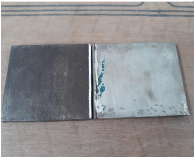
Fig. 2 Base Material (Left) Mild Steel1090, and (Right) Stainless Steel304
