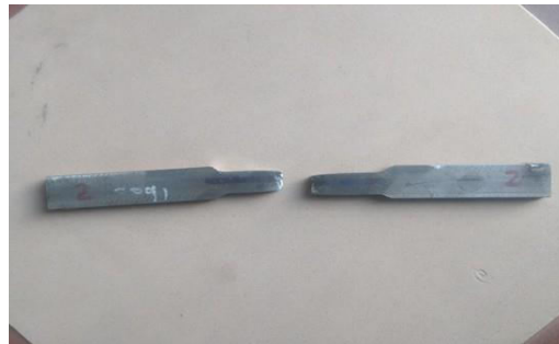
Figure 3: Specimen after Tensile Test
