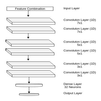
Fig:Graphical representation of feature-level combination.
