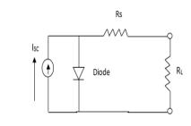
**Figure 3.7:** Equivalent circuit used in the MATLAB simulations
