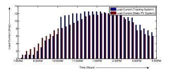
Figure 5.10 Variation in load current due to one degree of freedom (Y-axis tracking)5.4 CONCLUSION
