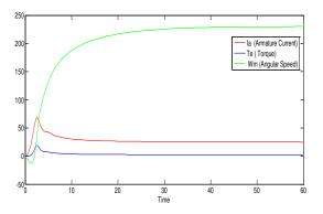
Figure 4.13 Simulation result of SWDC motor directly connected to PV module
