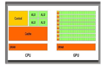
CUDA is NVIDIA's parallel computing architecture which enables dramatic increases in computing performance by harnessing the power of the GPU (graphics processing unit).The programmer can choose to express the parallelism in high-level languages such as C, C++, FORTRAN or open standards as OpenACC Directives. The CUDA parallel computing platform is now widely deployed with 1000s of GPU-accelerated Applications shown below.
