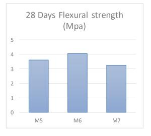
For each mix proportions, 3 beams were casted and tested after 28 days curing.
