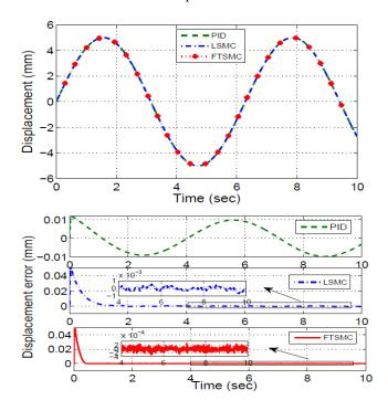
Fig. 5: The response curves for tracking a sinusoidal signal in the presence of disturbance compensation, (a) displacement, (b) Displacement error.
