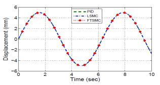
Fig. 3: The response curves for tracking a sinusoidal signal In the absence of disturbance compensation, (a) displacement, (b) Displacement error.
