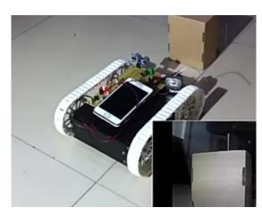
Fig -5: Ultrasonic obstacle detection
