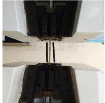
Fig -5: Bamboo Strip Tensile Test
