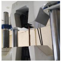
Fig -6: Bamboo Cylindrical Strip Tensile Test
