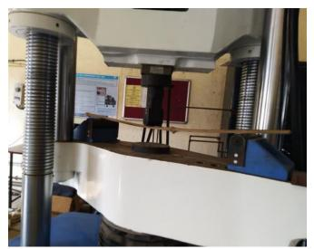
Fig -3: Bamboo Strip Bending Test
