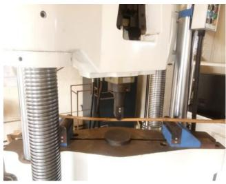
Fig -4: Hollow Cylindrical Bending Test
