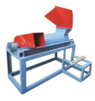
As the plastic material mixes and spins around within this lengthy transport tunnel, moisture is effectively dehydrated. Ending with a cyclone separation apparatus, where cool air is mixed in, residual moisture is further reduced. The cyclone separator is the last stand against any dust and fines within the material stream.
