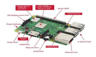
Raspberry Pi 3B+ module has 40 GPIO pins. It has 4 USB ports to connect keyboard, mouse, web camera and Dexter Er2 Robotics. HDMI cable used to connect the monitor. USB port is used to give supply to Raspberry Pi 3B+.
