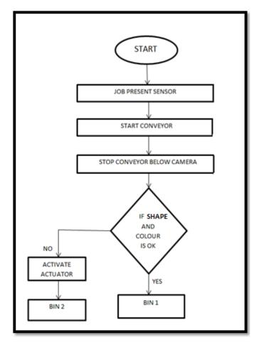
Here, when start button is pressed then conveyor motor will be started. By using proximity sensor, the conveyor motor stopped when object will come below the camera. Then the image of the object will be taken by camera for image processing. After that if the shape and colour of the object is OK then it will proceed to the end of the conveyor and then it will go into the bin 1. If shape and colour of the object is not OK then actuator will separate that object into bin 2.
