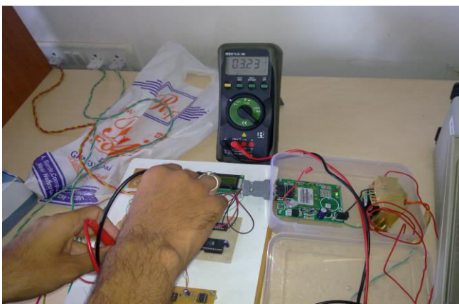
Fig -8: Output of I to V converter = 3.23 V
