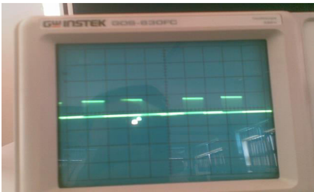
Fig -6: Output of zero crossing detector = 4.6 V
