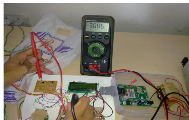
Fig -4: Output of amplifier stage = 3.086 V
