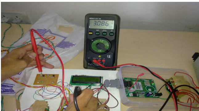
Fig -7: Input of I to V converter (I to V) = 3.086 V
