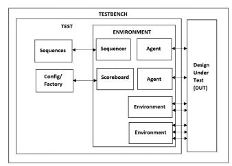
Fig -1: UVM Testbench Architecture
