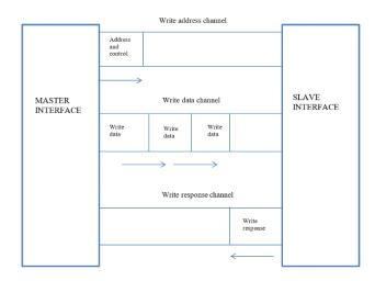
Fig -4: AXI WRITE FLOW
