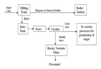
Fig. 1. A schematic diagram of formation of pressmud waste in sugar mill.
