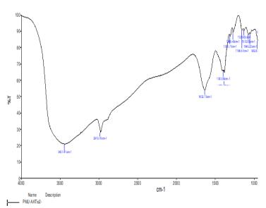
Fig : 2 FTI spectra of the  $SiO_2$ -TiO<sub>2</sub>-ZnO Nanocomposites
