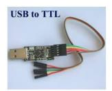
and microcontroller. PC will send information of the processed image to the microcontroller using USB to TTL cable. The cable is easiest way ever to connect to your microcontroller/Raspberry Pi/WiFi router serial console port. Inside the big USB plug is a USB<->Serial conversion chip
