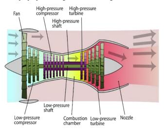
Fig -2: Working Principle of Jet Engine
