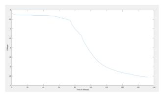
Discharge curve for battery used
