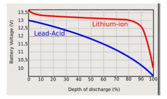
Due to non linearity in the dischrge curve of lithium ion battery it is not possibble to to estimate SOC using OCV method. Also this method of estimation is offline that is we can not estimate real time SOC of any battery being used.
